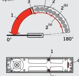
NOTE: Clockwise turns create a longer delay time with a slower closing speed. Turning valve completely clockwise creates hold open and eliminates delayed action.
