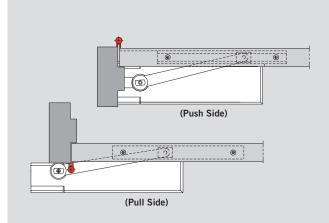
Track is surface applied to the door for U.L. fire door listing.
