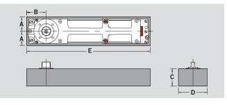
Maximum door widths and recommended sizes shown are for average conditions. If there are unusual site conditions, e.g. high or exceptionally heavy doors or wind pressure, the next stronger spring size should be selected.
