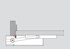
Track is surface applied to the door for U.L. fire door listing.
